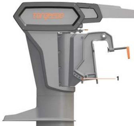
Fig. 40: Securing cotter pin for trim rod
