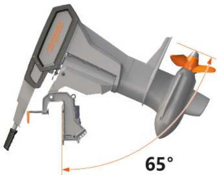
Fig. 55: Motor is tilted fully upwards
